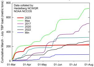
**Fig. 2.** Cumulative TBP loads for the Maumee River (Waterville, OH). Each line denotes a different year. 2023 is in red: the solid line is the measured load to June 26th; light red shows the possible max. The July TBP load will have the greatest impact on bloom severity, and could push the bloom severity of the maximum value (4.5).
