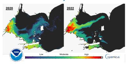
**Fig. 4.** The maximum bloom severity in 2020 (Aug. 21-31) and 2022 (Aug. 10-19). 2023 may be similar to 2020 and smaller than 2022. Bluish-green to dark blue indicates low cyanobacterial concentrations. Sandusky Bay has a different type of cyanobacteria that typically does not form scum.
