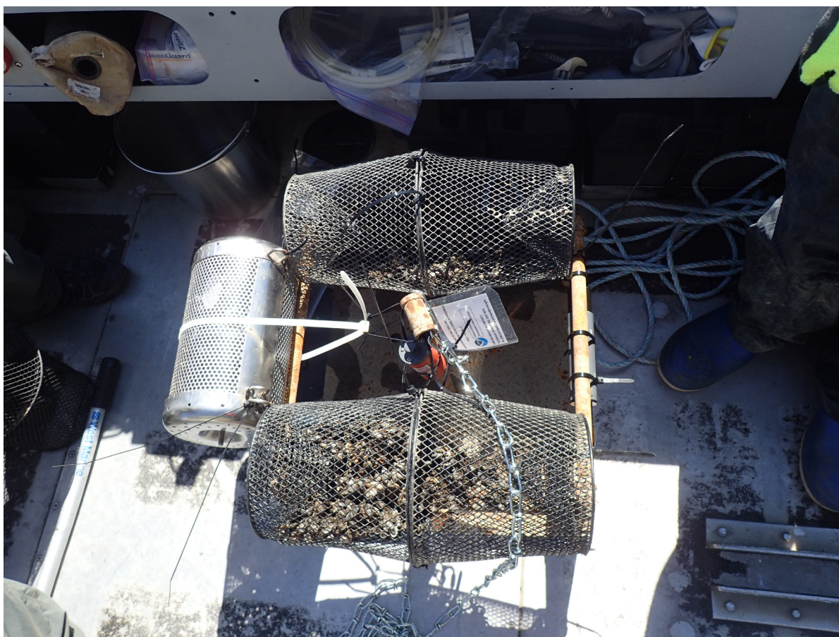
Figure 2. Multi-indicator mooring apparatus with mussels, polar organic chemical integrative sampler (POCIS) and data loggers.
