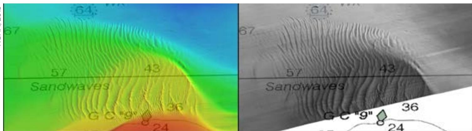
**ACOUSTIC PRODUCTS** collected by the NOAA Ship *Thomas Jefferson* depicting a sand wave field. Color shaded bathymetry (left) and backscatter intensity (right).
