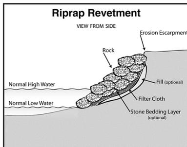
**REVTMENTS** are sloped structures built against the shoreline to absorb wave energy and prevent erosion. Building materials include rock, concrete and oyster shells. These structures are long lasting and can be combined with marsh grass plantings. The riprap provides habitat for some aquatic species. Revetments should be placed as far landward as possible to conserve the intertidal zone.
