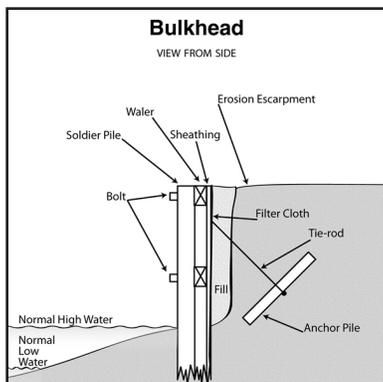
**BULKHEADS** or **SEAWALLS** are hard, vertical structures and are a common shoreline stabilization structure. Because they reflect, rather than absorb, much incoming wave energy, scouring of adjacent sediment can occur. Reflected wave energy may not allow marsh vegetation and aquatic organisms to thrive in front of bulkheads. Bulkheads may reduce the amount of sediment and nutrients flowing into the marsh.
