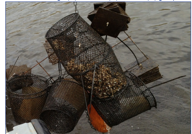
Fig 3. Sampler with three indicators- caged mussels, PEDs and Hester Dendys on board
