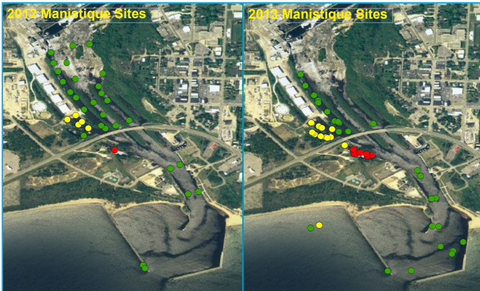
Fig 6. Caged mussel results from 2012 and 2013 Manistigue assessment. PCB concentrations were clustered into low (●; 286-3035 ng/g lipid), medium (●; 3036-14751 ng/g lipid) and high (●; 14752-39315 ng/g lipid) using Ward's hierarchical cluster analysis.
