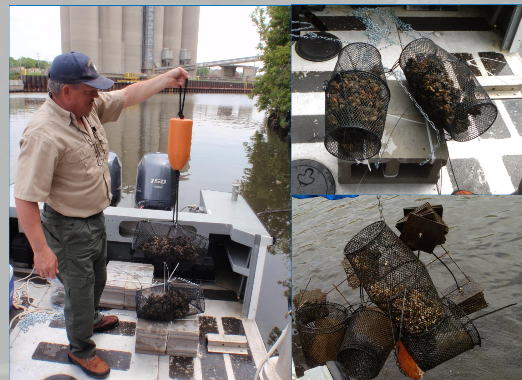
Figure 2. Caged mussels are deployed in minnow traps and placed on cinder blocks or a mooring that suspends them approximately 12 inches off the sediment. Mussels have been deployed with Hester-Dendy, Polyethylene Devices (PEDs), and Polar Organic Chemical Integrative Samplers (POCIS).
