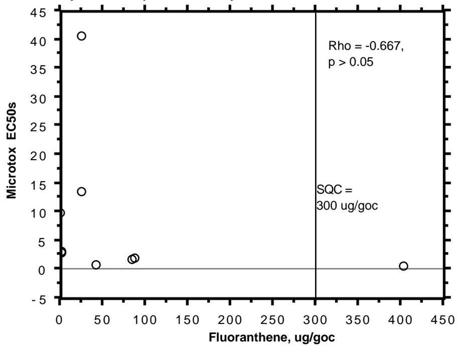
**Figure 76. The relationship between Microtox™ EC50's and the concentrations of fluoranthene (ug/goc) in samples from Bayou Chico and Apalachicola Bay.**
