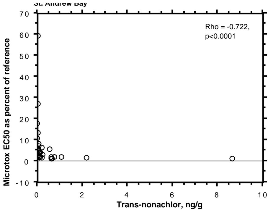
Figure 86. Relationship between microbial bioluminescence (Microtox EC50's) and the concentrations of trans-nonachlor in St. Andrew Bay sediments.
