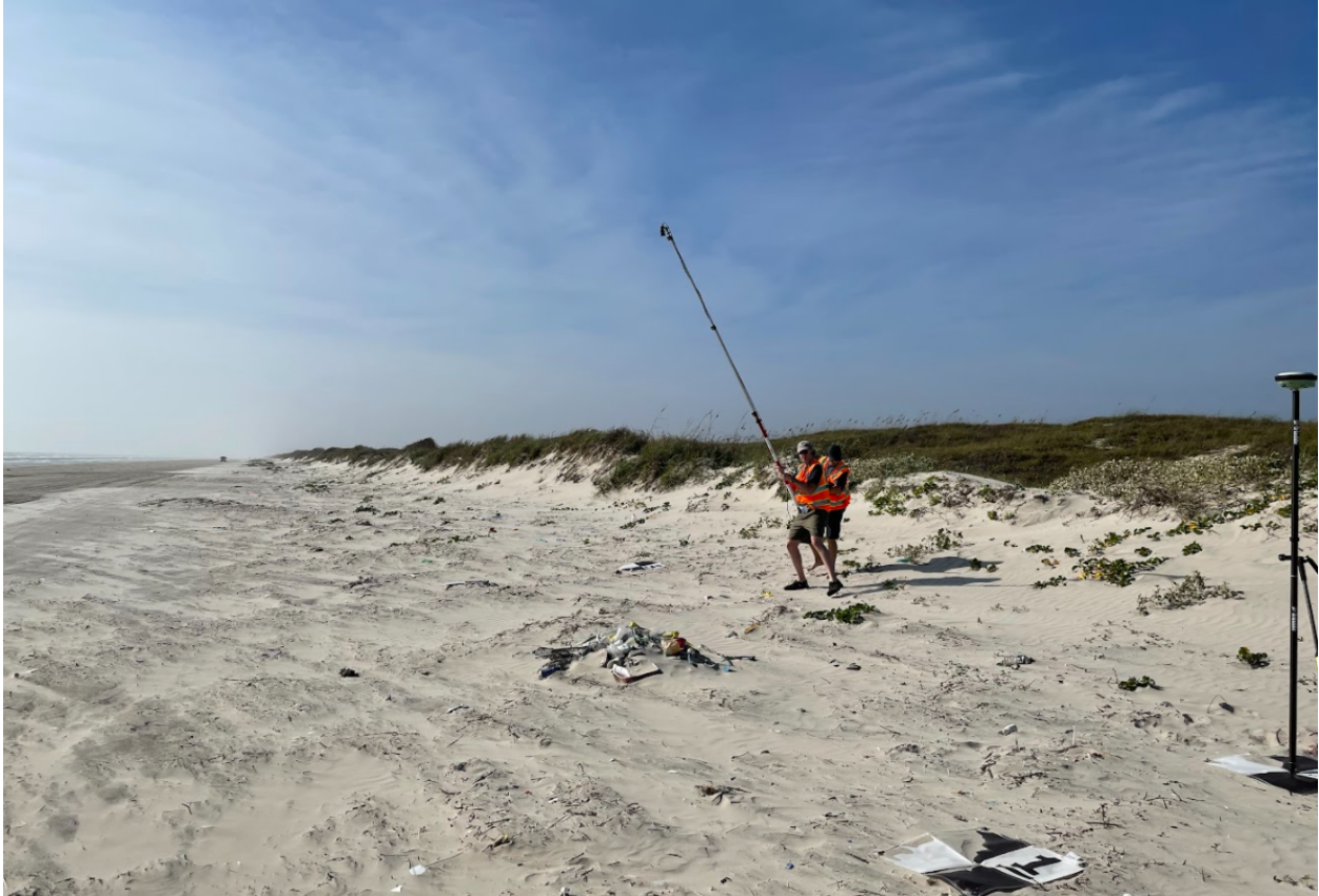
Figure 4: Pole-mounted PI camera acquisition at Padre Island.
